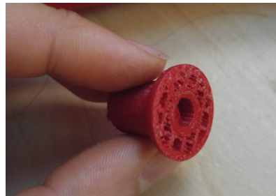
Fig U2: The bottom of the Red knob that didn't print correctly
