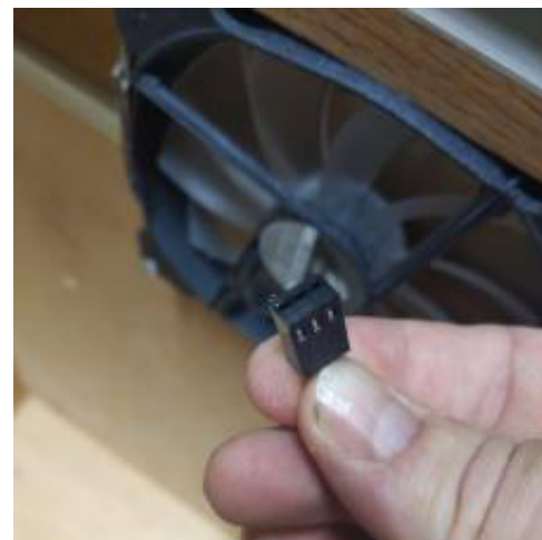
Fig U4: Keith's awesome fan solution, that terminates to a standard motherboard fan power jack
